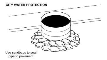
Using corregated metal pipe (CMP) over utility hole to isolate sewer line or prevent contamination of water system.
