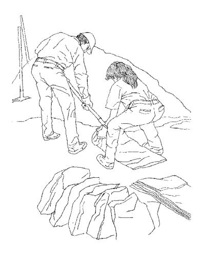
Figure 1: Proper sandbag filling
