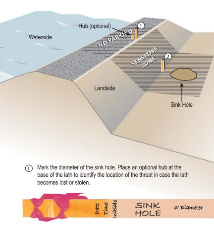
Measured from the levee toe, mark the distance to the edge and to the center of the sink hole. Place this lath when sink hole is located far from toe.
