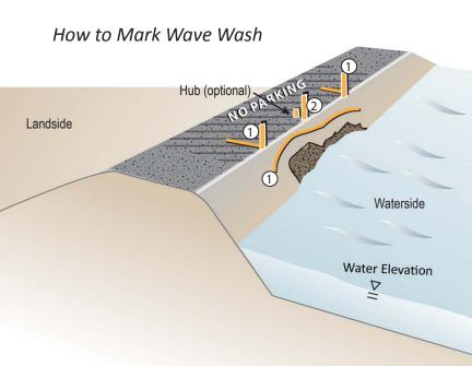
1 Place one lath at the beginning of the area experiencing wave wash and one at the end. Mark each lath with an arrow pointing inwards toward the location of the threat. Add lath as the threat grows (do NOT remove old lath). Paint can be used as an alternative to placing lath.
