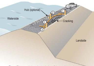
Place one lath at the beginning of the cracking and one at the end. Mark each lath with an arrow pointing inwards toward the location of the threat. Mark the largest width and depth of cracking. Add lath as the threat grows (do NOT remove old lath). Paint can be used as an alternative to placing lath.
