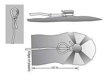
Figure 11: Plastic Tie-Down Buttons
