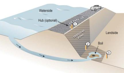
Mark the diameter of the boil and the approximate flow rate. Place an optional hub at the base of the lath to identify the location of the threat in case the lath becomes lost or stolen.
