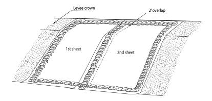
Figure 14: Emergency spillway using plastic sheeting and sandbags
