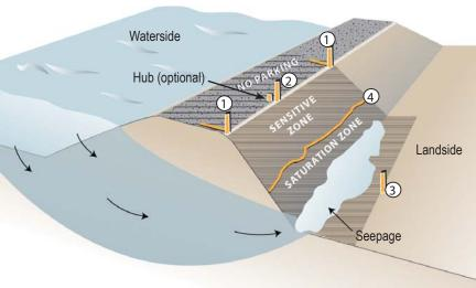
Place one lath at the beginning of the ponding location and one at the end. Mark each lath with an arrow pointing inwards toward the location of ponding. Mark whether the water appears to be clear or carrying material. Add lath as the threat grows (do NOT remove old lath). Paint can be used as an alternative to placing lath.
