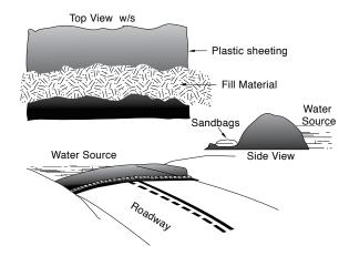
Figure 4: Temporary levee
