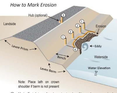
Mark offset distance from levee toe to edge of berm where no erosion has occurred – shows "normal" bench width and the extent of erosion. Place additional lath at levee toe as threat grows (do NOT remove old lath).
