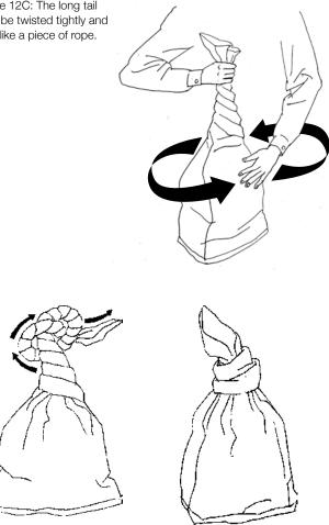
Figure 12D: Tie an overhand knot (pretzel knot) as low as possible on the bag.
