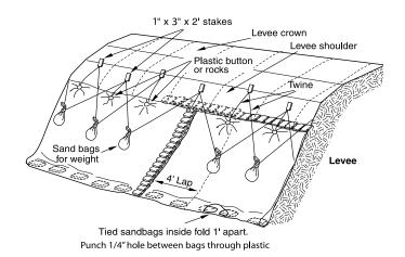
Figure 10: Wavewash Protection
